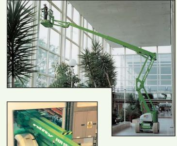
With more outreach than any other machine in its class and a base width of only 1.50m, the HR15N in one of the most effective and versatile self-propelled platforms available.
