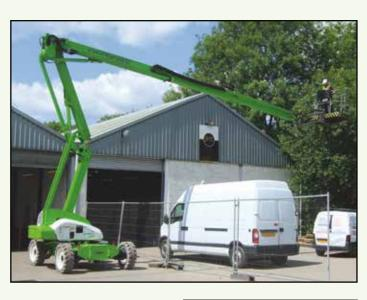
The **HR21 Hybrid AWD** also incorporates **ToughCage** and **SiOPS**<sup>®</sup> technologies. A tough impact resistant composite base and larger cross-section steel give the **ToughCage** strength and durability, while **SiOPS**<sup>®</sup> offers additional operator protection.
