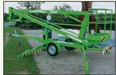
To save time and energy when setting up, the 120 is also available with a hydraulic outriggers option.
