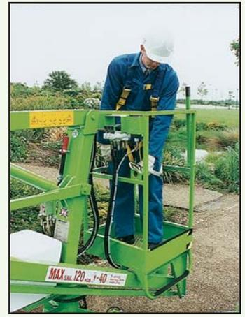
The Nifty 90 has a telescopic axle allowing it to pass through a 0.75m (2ft 6in) opening and a harness point in the platform for operator safety when working.
