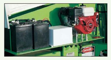
The Bi-Energy power option improves utilisation for the TM40 by allowing operation in discreet and fume free environments or for extended periods where no external power source is available.
