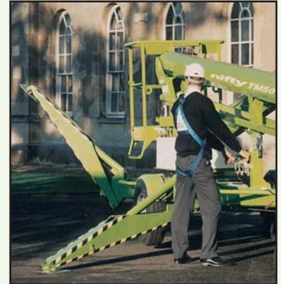
Fully proportional hydraulic outriggers make setting up and levelling quick and easy even on gradients.
