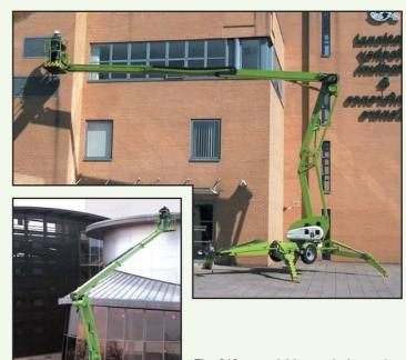
The 210's special boom design makes it ideal for working near walls or buildings. A single control allows its platform to move vertically while remaining parallel to the job, saving time and improving efficiency.
