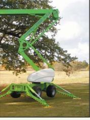
The extra manoeuvrability available from the 4 wheel steer option coupled with the special "Turf Tyres" make the 210SD ideal for working on sensitive surfaces such as grass.
