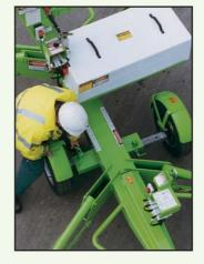
Retractable axles allow the Nifty 120 to pass through a 1.10m (3ft 6in) wide opening.
