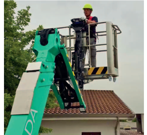
Active hydraulic jib and basket rotation \pm 62^\circ : complete placement on working site in any condition.
