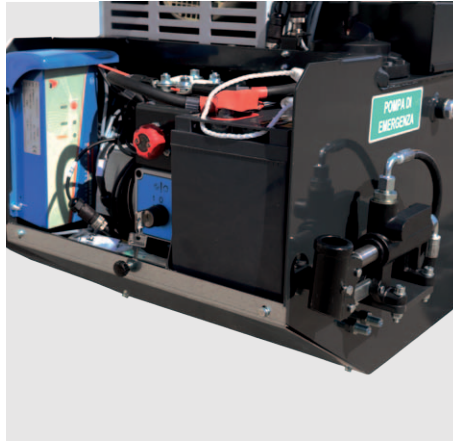
Manual emergency pump and compartment hosting the battery and the control of emergency electro-pump and battery connection.
