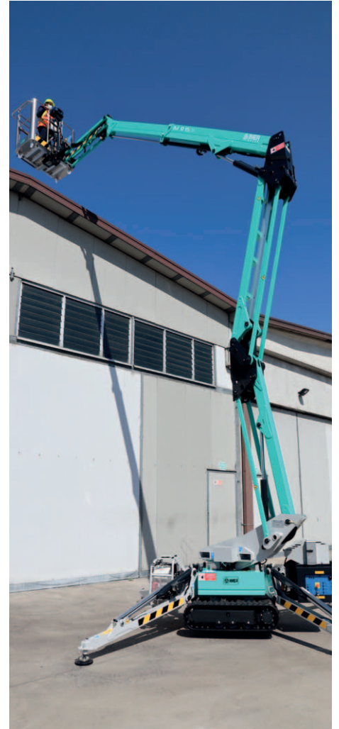
The Up & Over height of 7 m allows to easily overcome obstacles at height.
