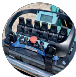
The control panel is removable and can be used by the operator even on the ground. In this case, the traction and stabilization movements are enabled both in the radio-controlled version (up to a distance of 10 m) and in the wire-controlled version (with 5 m coiled cable).
