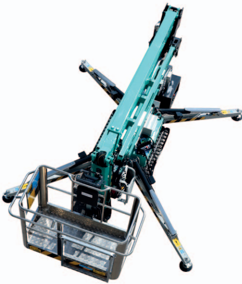
45° stabilization in limited overall outrigger footprint.
