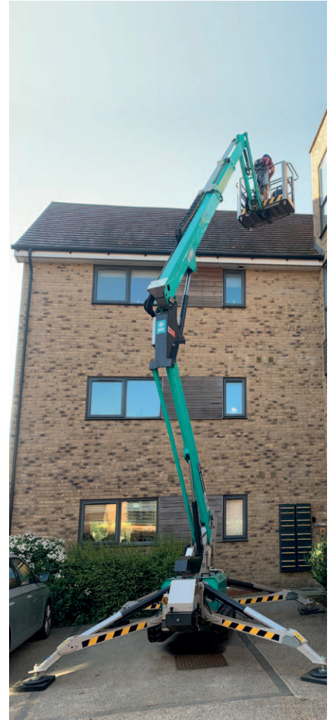
The articulated arm with active jib and the basket rotation \pm 62^\circ , together with the turret slewing 360^\circ (not continuous), allow the optimal positioning of the machine in any working situation.
