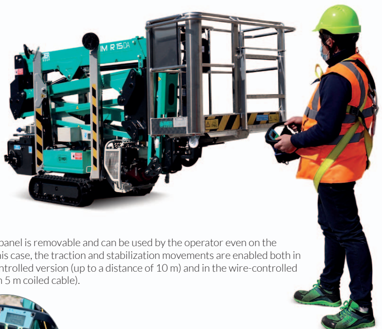
User-friendly control panel with external support to the basket.
