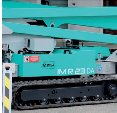
Hydraulically adjustable tracks width: more stability and traction to move around the building site or rough terrain.
