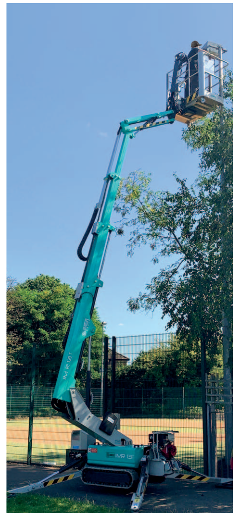
Automatic stabilization in work position ensures maximum easiness of use and safety.
