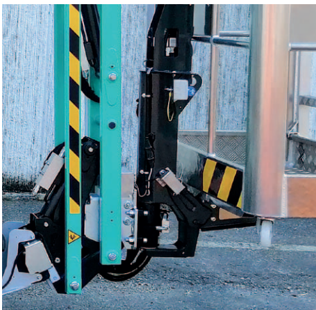
Compactness of the jib assembly hosting the load cell and basket rotation.
