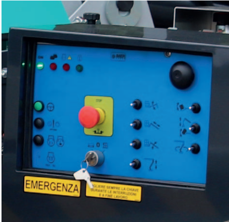
Ground control panel.
